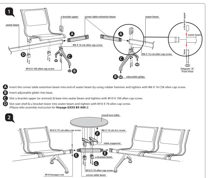
(E) Insert corner table beam into 2 different seater beam and tighten with M10 X 75 csk allen cap screw and M10 hexagon nut.
